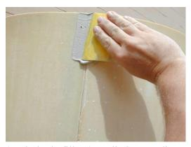
4) Mix body filler (supplied) according to manufacture's instructions and apply to joint. Make joint wide enough to make a smooth radius.
