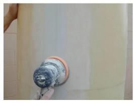
6) Sand cured body filler. For best results, use care when sanding to maintain an even radius. Finish with 120 grit paper.
