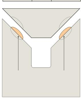
Plan view of "V" cut - shows jointer biscuit recessed into edge
